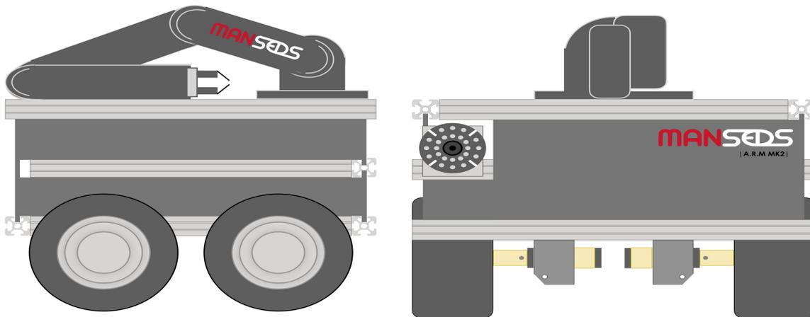
The rover will be built to have 3 separate layers joined together with struts of different lengths, the rover will also have a robotic arm mounted on the 2nd layer, with the base completely submerged below the 1st layer, providing a large range of motion for the arm.
