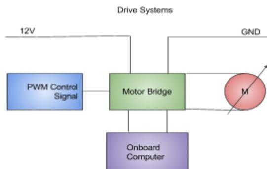
The electronic motors are controlled using a PWM/Servo hat. This configuration requires motor bridges, and the PWM signal generated by the Adafruit PWM/Servo hat using code from the raspberry pi then dictates whether the motor will rotate clockwise or anticlockwise using these bridges.
