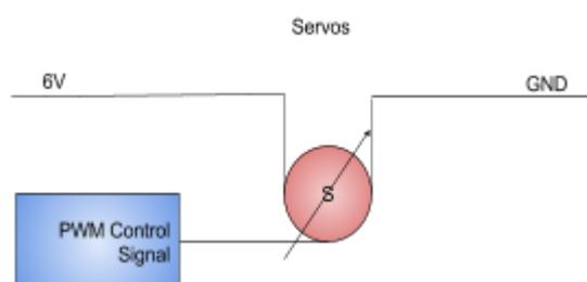
The collection system chosen is a robotic arm connected to an excavator as the effector. This is a more precise but more complicated collection system. The precision is provided through the control of six degrees of freedom, which requires relatively complex control code to drive several electronic actuators. Each joint will have a servo controlled via pulse width modulation (PWM),
